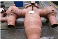
Obr. 10 Kontrola svaru ventilu Fig 10 Inspection of welds
