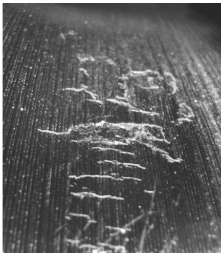
Obr. 20 Vada (obr.19) během soustružení Fig. 20 The defect (Fig.19) during turning
