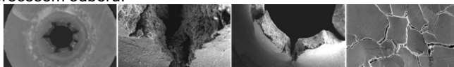
Obr. 2 Detail trhliny ve vzorku po SPT, Detail of the fracture in the sample after SPT
