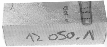
Obr. 3 Vzorek oceli s laserově zakalenou stopou Fig. 3 Sample of the tool steel with hardened track
