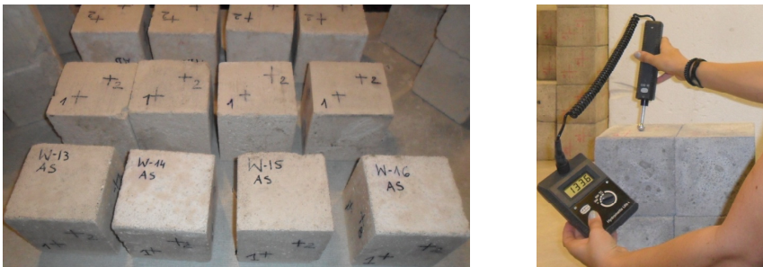
Fig. 1. View of: a) lime mortar cubes prepared for testing, b) lime mortar tested using dielectric technique.
