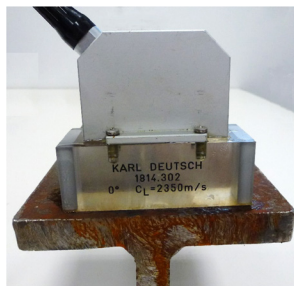
Figure 3: Weld inspection on a T-joint with 5 MHz and 64 elements probe.
