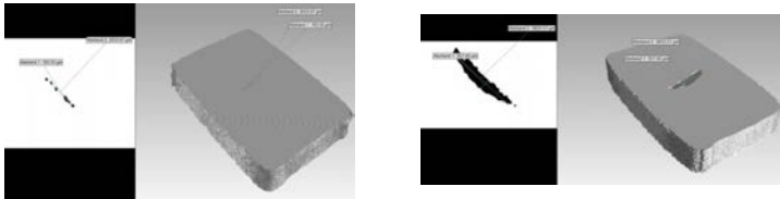
Fig. 3: Circular defects of diameter 5 mm and maximal thickness of 200 (left) and 500 (right) \mu\text{m} , respectively. Cross sections of defects are shown on metallography of samples similar to #1 and #4.
