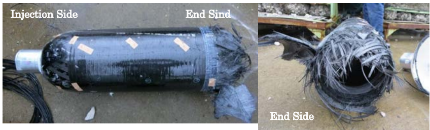
Fig. 3 Picture of pressure vessel after broken
