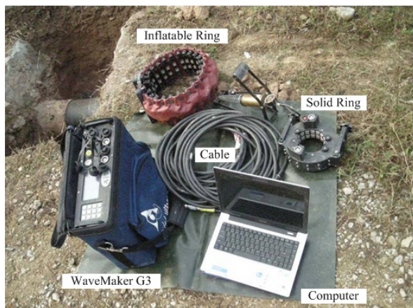
Fig.2 The photograph of the guided wave testing system WaveMaker G3.
