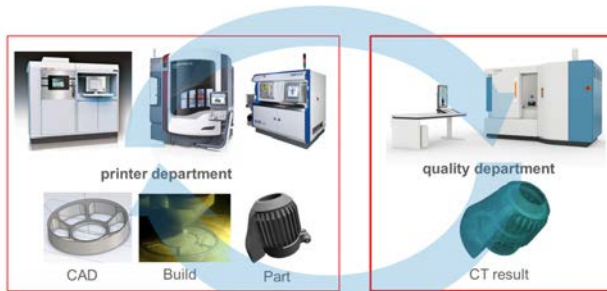
Figure 8: CT as a tool for process optimization.
