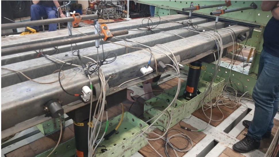
Fig. 3 – Location of acoustic emission sensor
